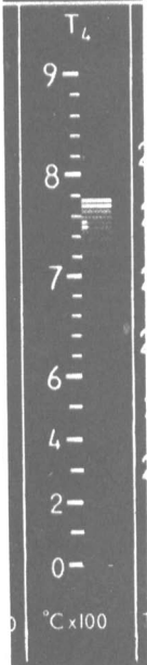
Figure 3.16 LED vertical scale display.
